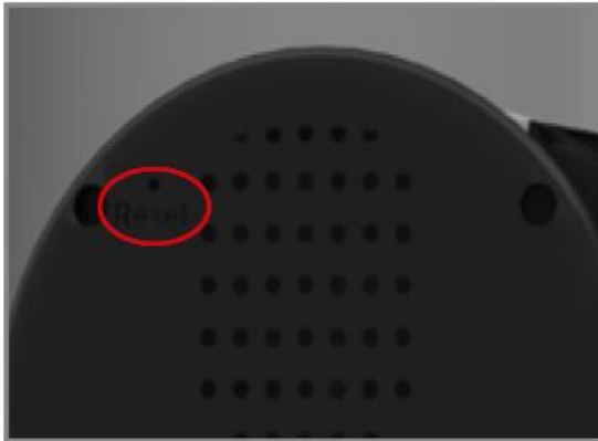
For Cube camera Reset button is at the back of the camera
